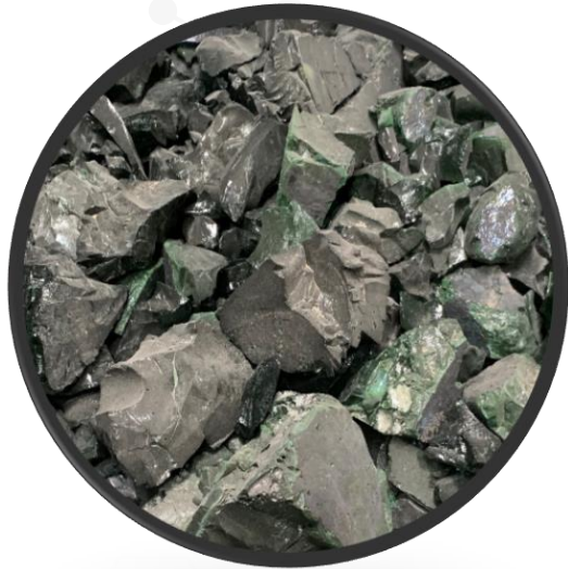
Slag: Generally borosilicate, vitreous matrices.
