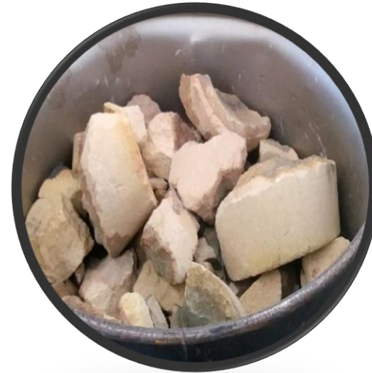
Spent Crucibles: Silicon-carbide, graphite, fused silica, or fired clay.
