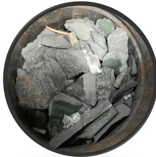
Slag: Generally borosilicate, vitreous matrices.
