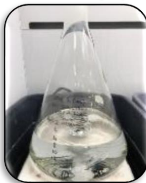
Sn dissolved in HCl and H 2 O OK on ICP-OES
